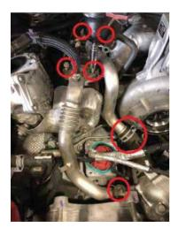
In the supplied parts bag of the Cooler Upgrade Kit locate the Billet Plug with 0-ring and apply grease to the 0-ring, then install the plug into the coolant port on the thermostat housing just in front of the passenger side intake port. Fasten with the OEM bolt that was removed in the previous step.
