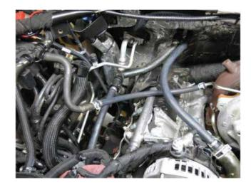
Locate the Bridge Block Off Plate Supplied 8mm flange head bolts, and gasket. Install block off plate on to Y-Bridge and torque flange bolts to 25 ft lbs.
