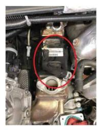
Then remove the five 13mm hex head bolts that hold the EGR cooler to the engine and remove the cooler assembly.
