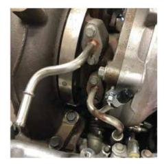
The above picture also shows the location of where to install the supplied<sup>1</sup>/<sub>4</sub>" Silicone cap and hose clamp to block off the no-longer-needed coolant port on the coolant supply line (lower) to the turbo center section.
