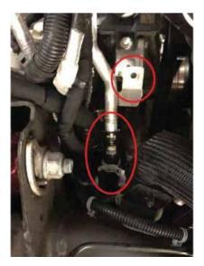
This hardline also has a smaller diameter line welded to it that feeds coolant to the urea Injector, these small rubber lines also need to be disconnected from the line so that it can be removed completely. Here is the assembly removed;
