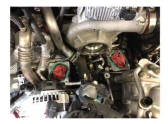
Now remove the heat shield on the shorter EGR hot side pipe connecting the Lower EGR valve to the Upper EGR valve, and then remove the four 13mm hex head bolts holding the pipe on and remove the pipe.
