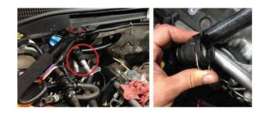
At the bottom of the hard line just in front of the upper control arm, remove the hose from the hard line and leave the spring clamp on the HOSE it will be reused. Remove the bolt connecting the hardline to the engine also.
