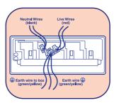
Locate conductors into correct terminals. Ensure that all bare conductors are housed in their respective terminals before tightening the terminal screws.
