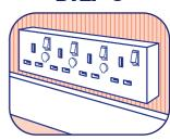
Fit the three round screw cap covers into place Wipe clean with a dry cloth. Switch on at the mains.
