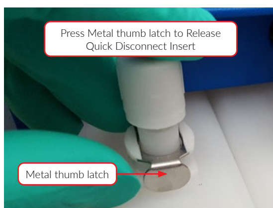
Figure 3.9 Releasing the Quick Disconnect Fittings
