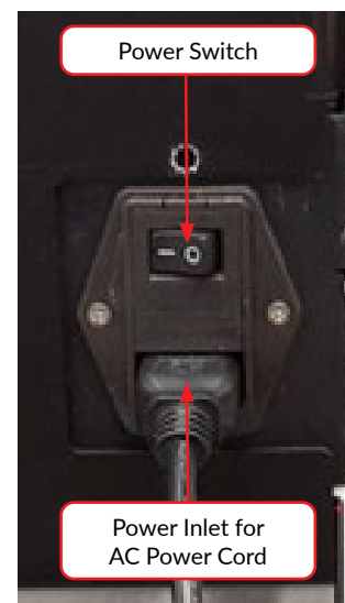
Figure 2.13 The power panel of the ML230 instrument
