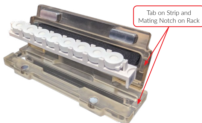
Figure 3.10 Assembling microTube 8-strip into Rack
