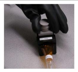
4. Release the cylinder. Strike the top of the cylinder with the Covaris impactor as demonstrated below to pulverize the sample.
