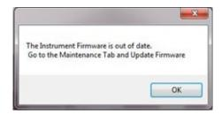
Figure 6.14 Firmware out of date alert
