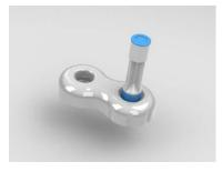
7- Unscrew the tube body leaving the screw-cap containing the sample in the stand.Recover the sample from the screw-cap. You may tilt the stand to aid sample recovery.
