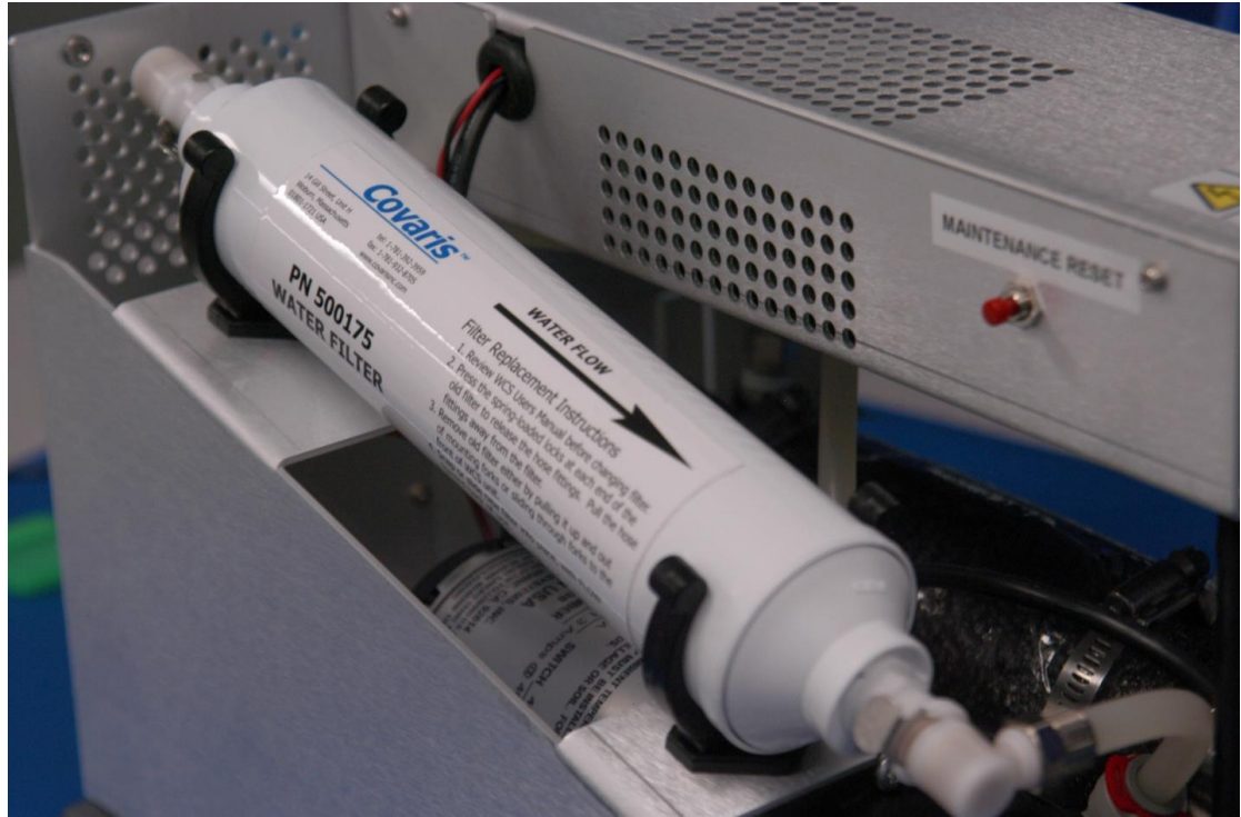
Figure 10 – Filter cartridge orientation
