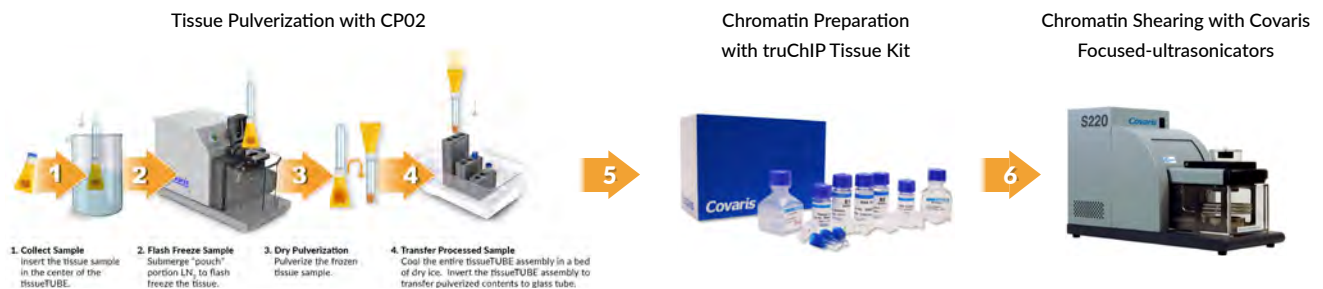
Figure 3. Processing of tissue samples with the cryoPREP dry pulverizer enables fast and easy processing without sample heating or cross contamination. After cryofracturing, standardized chromatin preparation is performed using Covaris truChIP tissue kit followed by Chromatin shearing on a Covaris Focused-ultrasonicator such as the S220.
