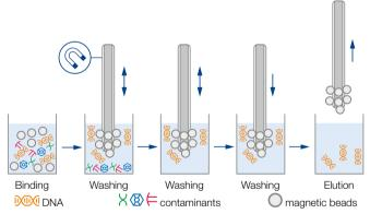
Binding of DNA to the NucleoMag® B-Beads is achieved by the provision of Binding Buffer MB2. After magnetic separation, the NucleoMag® B-Beads are washed to remove contaminants and salts using three different wash buffers (MB3, MB4, and MB5). Highly pure genomic DNA is finally eluted under low ionic strength conditions in a slightly alkaline elution buffer (MB6).
