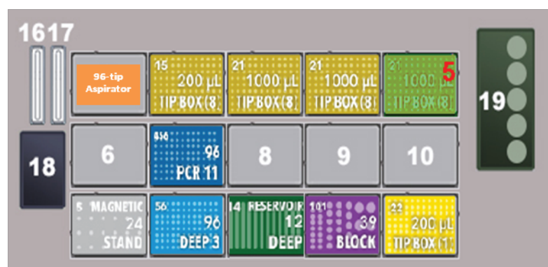
Figure 2: The deck layout of the VERSA 1100 used to automate the NucleoMag® Blood 200µL genomic DNA extraction workflow. Position #17 is the liquid waste disposal site, #18 is the tip disposal chute and #19 is the ReagentDrop bulk reagent dispensing system that is part of the robotic pipette head.
