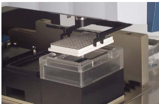
Figure 1: The internal plate handler iSWAP places the NucleoFast® 96 PCR plate on the vacuum chamber of the MICROLAB® BVS (Basic Vacuum System), which is positioned on the MICROLAB® STAR deck.
