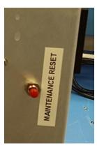
NOTE: The MAINTENANCE indicator will remain illuminated if the UV lamp has not been correctly plugged in or is not operating.
