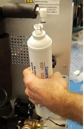
4. Install the replacement filter by pressing it down into the plastic grips, taking care that the flow arrows point towards the bottom of the WCS 2.0 cabinet. Reconnect the fittings as originally found by pressing them into each Quick Connect socket until they snap securely.
