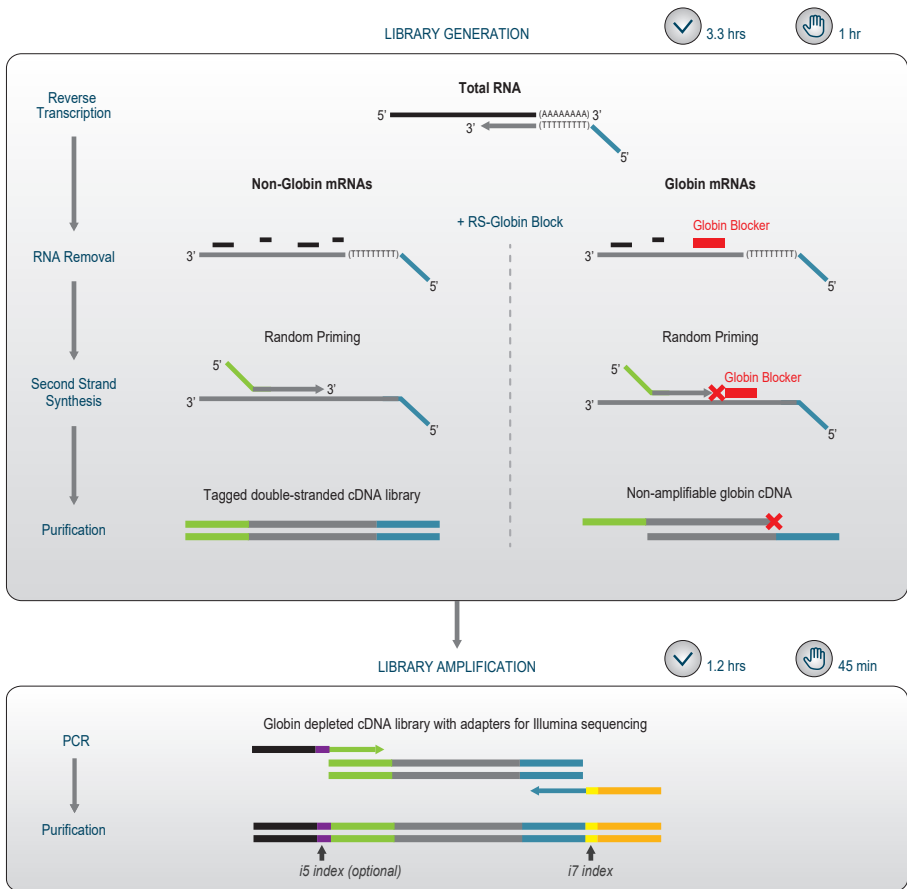
Figure 1. Schematic overview of the QuantSeq workflow using Globin Block Modules for globin depletion. Whole blood total RNA contains a mixture of both globin and non-globin mRNAs, which are both reverse transcribed by oligo(dT) priming during first strand synthesis. The RS-Globin Block (RS-GB ●) solution is then added instead of the standard RNA Removal Solution (RS ○). Following RNA removal, the Globin Blocker oligos bind specifically to globin first strand cDNA downstream of random primers and block globin second strand cDNA synthesis. After second strand synthesis, the sample will contain both non-amplifiable globin cDNA fragments and tagged double-stranded cDNA library fragments for non-globin mRNAs. During PCR, only the non-globin library fragments are amplified to add full-length adapters and indices for Illumina sequencing.
