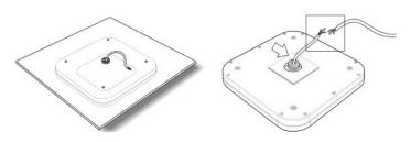
1. Drill [4] small holes 10.55" QC Using this template. At the centre of the 4 holes, also cut a notch on the ceiling to allow the wiring from the light to be powered with the AC Power Supply cable. Minimum notch size is 1.5" diameter hole. (As long as there is access to
