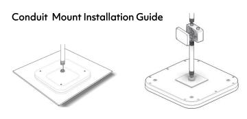
1. The back side of the light has a conduit connector at the centre with the LED Driver Input cable sticking out. This luminaire can be installed by simply threading a 3/4" conduit (conduit not included) to the back side. This can be done once the light is flush to the ceil-
