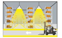
When motion is detected, the sensor will switch on the light to 100% brighteness.
