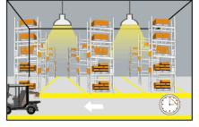
After elapse of hold time, the sensor dims the light at the present low light level if no motion is detected.
