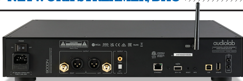
ABOVE: Wired and wireless Ethernet, USB-B (computer) and USB-A (external drive) inputs are good to 768kHz/DSD512 and are joined by optical/coaxial digital outputs (192kHz/24-bit) plus single-ended (RCA) and balanced (XLR) analogue outputs
