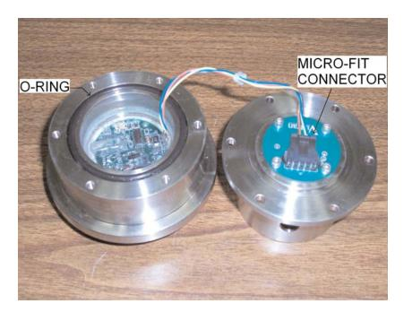
From the replacement kit remove the replacement sensor 'O'-Ring & package of grease. Grease the 'O'-Ring and place it in the groove. Attach the Micro-fit connector to PC board on the new adapter.
