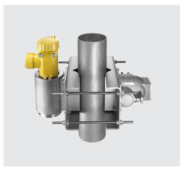
The truck-mounted version utilizes a universal bracket system to permit installation on a variety of pipe sizes. It features a detector background radiation shield to minimize errors associated with reflected radiation. These errors are caused by changes in other vehicle proximity from job-to-job.
