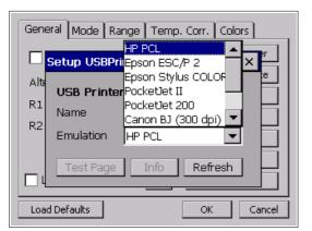
Certain external USB Printers can be connected. Select the desired printer to print results. Printers not listed are not supported.
