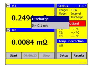
After storing the last measurement the instrument turns off the output Current, stops the measurement and automatically discharges the transformer until the test object is safe.
