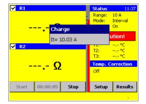
The heat run timer must be started the moment that the heat source is switched off from the test object.
