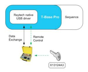
Sequence is an existing Add-On to control Raytech devices and doing complete transformer measurements in a free programmable measuring process, including winding resistance and turns ratio measurements.
