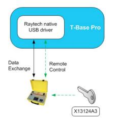
The T-Base Pro remote option of Raytech devices can be unlocked by entering a license key.
