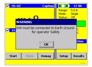
If the ground warning message is enabled, it will be displayed at every boot-up of the instrument and the message must be acknowledged to continue.
