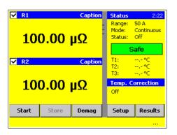
2. Select the Test Current: press Range or Setup / Range
