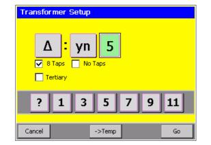
Confirm with OK to set (e.g. 8) Taps. View the number of Taps in this Transformer setup screen.
