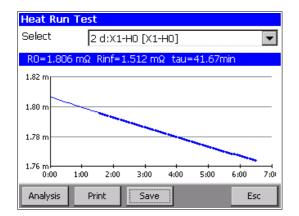
You can Print the Graph with the approximation or Save the calculated values to the corresponding results.
