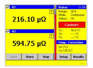
The "T" in the measuring channel box shows that the displayed resistance value is corrected. In this example it is corrected to 25 °C using Tk of Copper and referring to Temperature probe 1.
