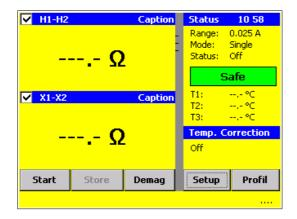
The Touch screen enables quick navigation by pressing directly on the screen. e.g. if you would like to change the current range, press on the text "Range" and the Menu Range will open. This is a short cut step to the Range menu. Or access Range menu by going through the Setup menu.
