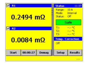
Although the measurement is finished, the timer continues to operate. This allows further measurements on other windings of the same transformer.
