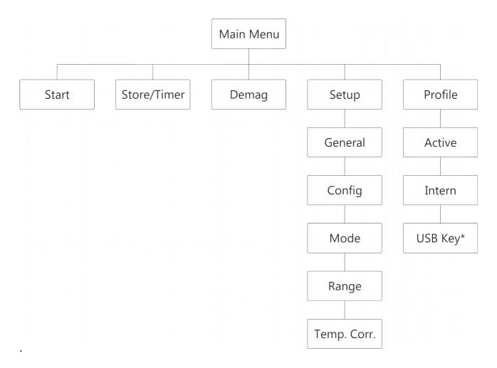
To use Profiles mode, as described in this chapter, turn it on in the Setup menu by selecting the check box shown in chapter 6 Operating Menu on page 28.
