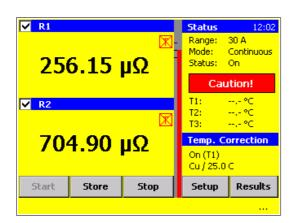
If the display shows a crossed Red T, the result is not corrected because a temperature probe is missing or not recognized by the system.
