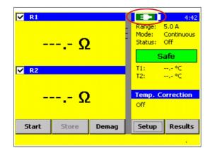
If you have the Battery Option, there is a Battery Symbol on the top of the main screen. It indicates the Battery status and the charging condition.
