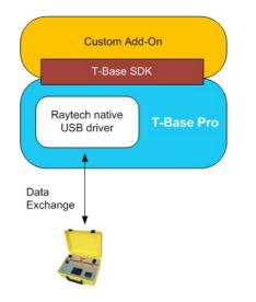
T-Base Pro is designed as an open platform. A <u>Software Development Kit</u> (SDK) to create custom Add-Ons easily is provided by Raytech.
