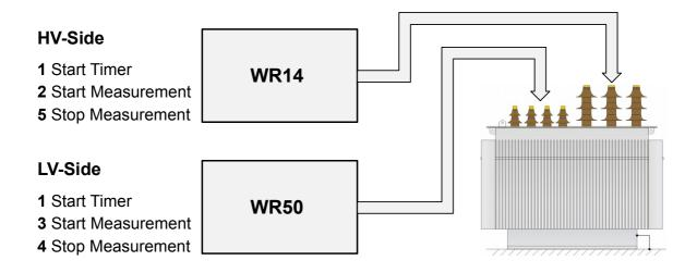
Now you can analyze the test results with the optional heat run test software to calculate the cooling curve. A description of this software can be found in chapter 7.2 Heat Run Test Software on page 70. Or you may export the results on a computer and analyze the data with our Software "T-Base Pro".
