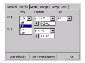
**WS**: Select the Winding System (1 Primary, 2 Secondary or 3 Tertiary side of the Transformer). The configuration of the appropriate winding can be made.
