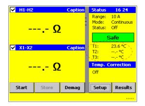
As soon as a temperature probe is connected, the value is displayed on the main screen and will automatically be stored to the correspondent resistance value.
