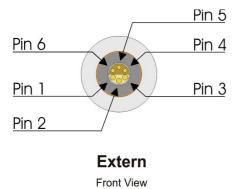
You can use pins 3 and 4 to connect an external Warning Light or Beeper to indicate a Dangerous condition. The function for these pins are the same as with the standard type, see chapter 9.1.3.1 Standard type on page 91.
