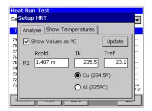
Enter the resistance value (Rcold) of the winding, the corresponding temperature (Tref) and the temperature coefficient of the conductor.
