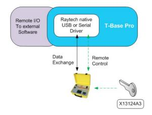
This is a basic Add-On provided by Raytech. It calls any program with a parameter on a PC. An XML file as return value is accepted.
