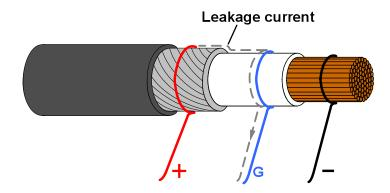
This diagram illustrates GUARD terminal used to prevent surface leakage on cable insulation from affecting a high resistance measurement.
