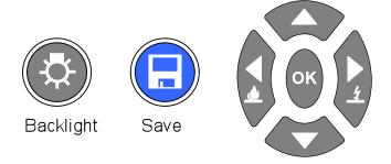
Four arrow buttons and OK facilitate adjustment and selection of settings, voltages and modes. Breakdown/burn modes are set using the left and right arrow buttons. Backlight and save functions are dedicated buttons. All models have backlight and the MIT525 and MIT1025 have the Save button.
