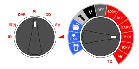
using the preconfigured voltage ranges on the central rotary switch or the V<sup>1</sup> user settable/lockable voltage range.
