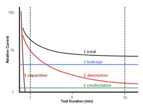
In the case of dry insulation, conductance current may be negligible and the leakage current may be low, in which case the absorption current will dominate the total current measured.
