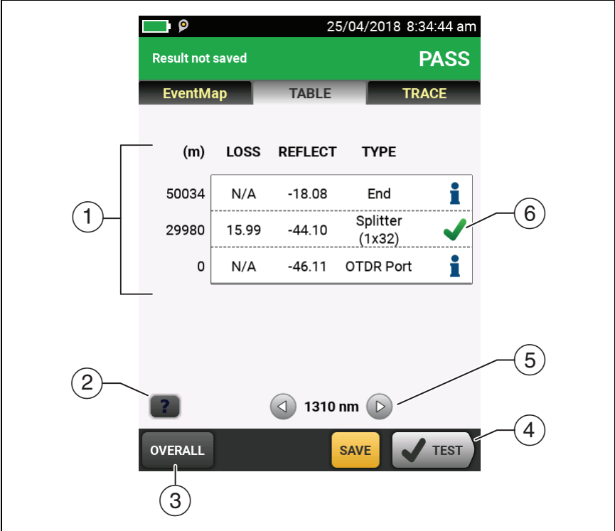
Figure 93. Event Table from an HDR OTDR Test
