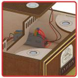
Insert the other sides of wires matching the black color wires to blue color switch and red color wires to yellow color switch. Once done, press down the switch to connect the wires.
