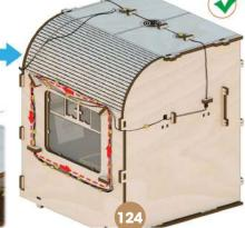
Follow the fixtures as shown in the graphics and use part (11) when necessary to hold the wires in place. Follow the direction of the wire fixture as shown in the red dotted lines and red arrows direction.
