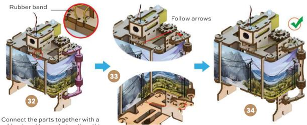
rubber band to create traction, this will help to ensure the film roll is always clammed between the 2 spindles. Please follow the arrows as shown in the graphics from Step 33-35.
