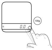
Place a 100g weight on scale and wait until the display shows '\_End\_'. Calibration is now complete!
