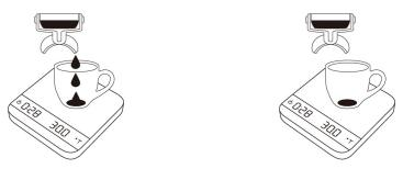
2. In all Auto Start Modes, if you do not operate the scale for 30 seconds, it will reset timer and perform tare operation.
