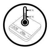
Avoid places where room temperatures are unstable. Room temperature above 40°C or below 15°C may result in weighing inaccuracy.
