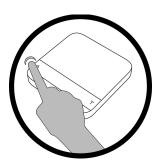
• Press button for 0.5 seconds to turn on the scale.
