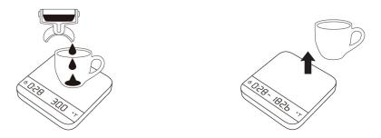
4. The scale will also display a previous stable weight that captures the coffee weight of the shot when you unloaded the cup.
