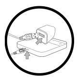
• To use AC adapter instead of the built-in battery, plug the USB cable into the Micro-B USB port located on the back panel of the scale.
