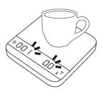
When the espresso flow stops with the timer running, the timer stops.
