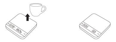
3. In all Auto Start Modes, the timer will stop when a negative weight (i.e. removal of cup) is detected.
