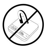
• Do not locate the scale near any equipment/instrument which contains magnets.
