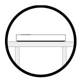
Select a work place that is stable, vibration-free and, if possible, a horizontal location for the weighing platform.
