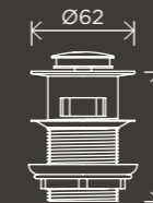
Basin Pop Up Waste 32mm - Overflow / Slotted
