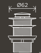
Basin Pop Up Waste 32mm - No Overflow / Unslotted
