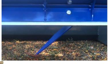
Once the roll is complete, position the roller horizontally just above ground level, and pull the release cable until the catch locks open.
