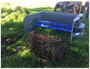
The Walters Fencing netting roller, in 1200mm and 1900mm capacity variants, is built to enable the rapid removal of old netting and hinged joint fences. Extra barbed and plain wires can also be rolled at the same time. Attaching to skid steer loaders or the front of a tractor, an integrated pick up arm lets you start the roll without having to manually attach wires. Once the roll is complete, the frame can be opened remotely by pulling a cable running from the manual lock to the vehicle cab.
