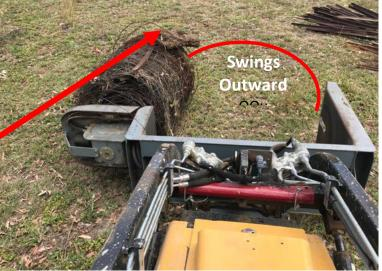
Continue reversing until the roll is completely clear of the centre drum, then crowd the loader to close the roller frame and lock up the drum core.
