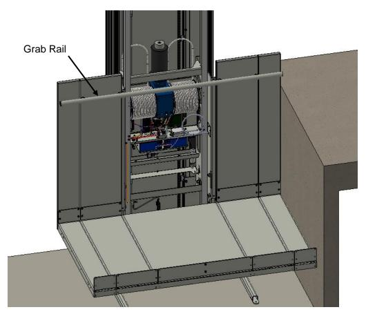
19. Install the Front Guard Panels with hardware as indicated.
