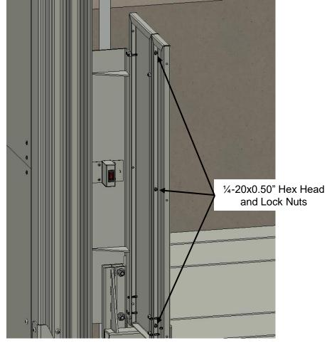
18. Install the Grab Rail utilizing the Rear Outer Guard Panel upper mounting hardware.
