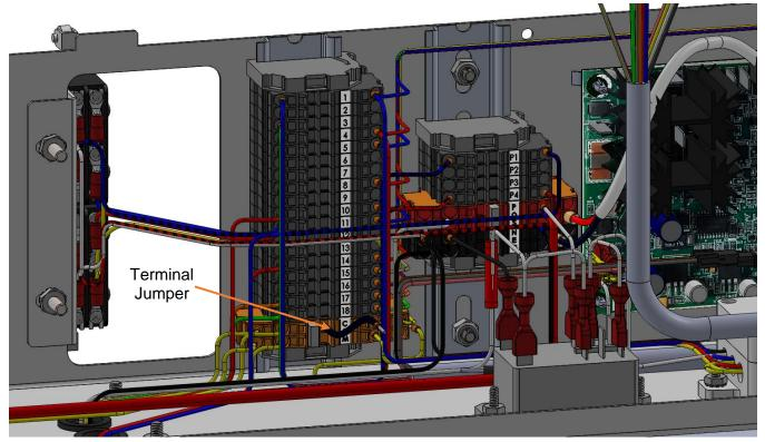
▲ WARNING! All jumpers must be removed from the Terminal Block before turning the lift over to the customer.
