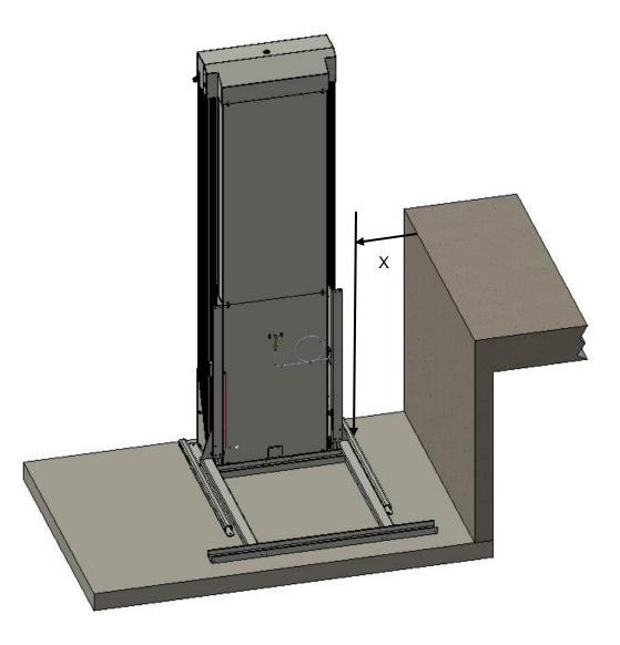
A The tower must be level and plumb in all directions, shim under the base plate as necessary.
