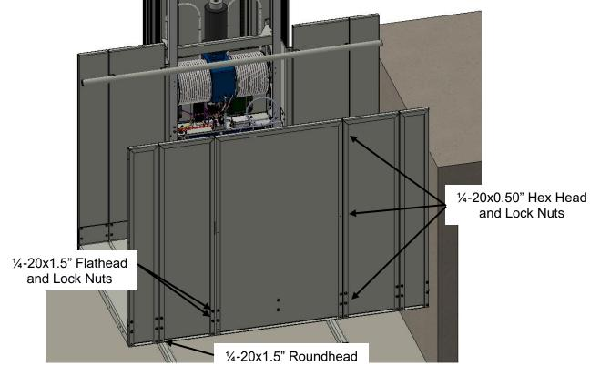
A Return to STEP 9 and all Platform fasteners assembled to this point should now be tightened sufficiently.
