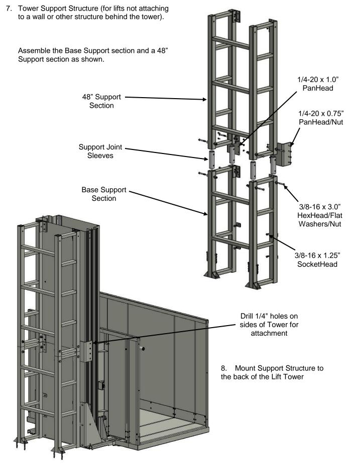
9. For taller lifts, continue with additional Support Sections to match the Tower Extension Modules.
