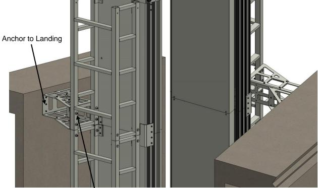
Drill mounting holes where needed
