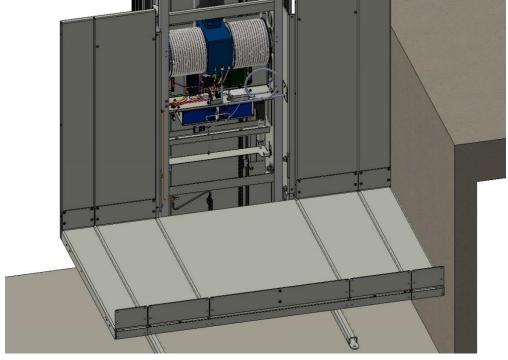
Also fasten the Rear Outer Guard Panels to the Extension Guard Panels.
