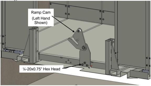
28. Install the Ramp Linkage Arm.
