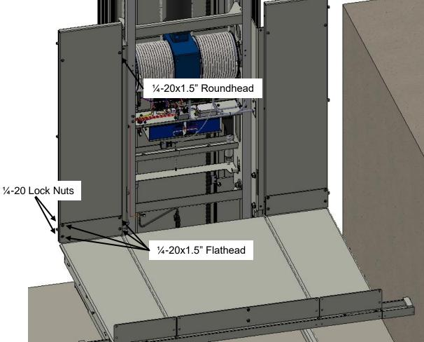
17. Install the optional Platform Extensions for a 54" or 60" long platform using steps 7 and 8.
