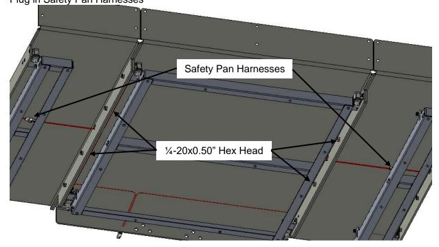
16. Install Rear Outer Guard Panels with hardware as shown.
