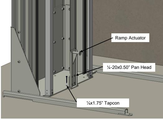
26. Mount the Folding Ramp to the end of the Platform (or Platform Gate if equipped).
