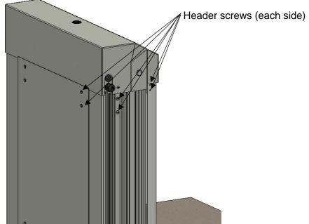
6. Using the provided hardware, join the Rail sections with the Inner and Outer Splice Plates. Also join the Front Cover Struts with the Front Cover Splices. Then reinstall the Sheave Header on top of the new Tower Extension Module.
