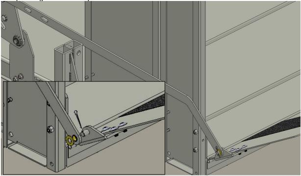
Fold the Ramp up manually until it stops to make sure the Ramp Cam is in the proper location before running the lift down onto the Ramp Actuator.
