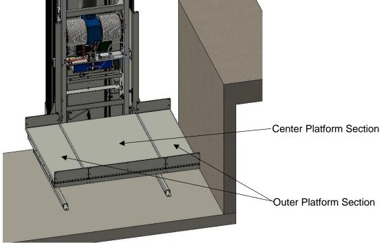
A It is recommended to assemble all Platform pieces together with the hardware only hand tight until all pieces are attached.
