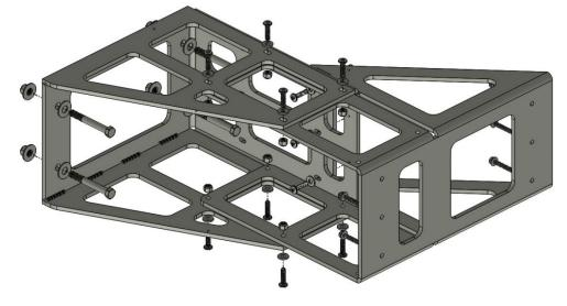
12. Depending on the lift height, drill 3/8" holes through the Tower Support Structure and attach the Landing Brace.
