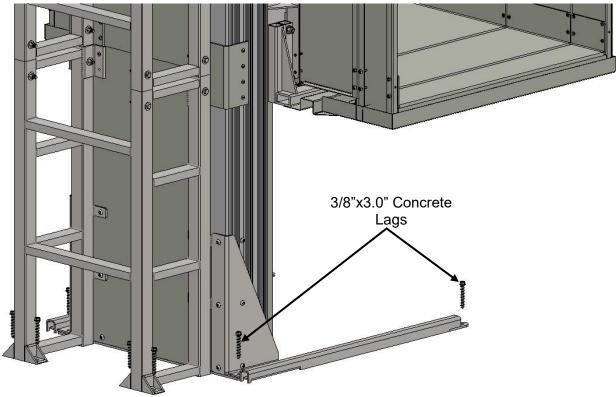
31. If installing against a wall or inside of a shaft, drill holes where needed to anchor into wall studs. There is a scribe line on the rails that are 16" apart to line up with the wall studs.
