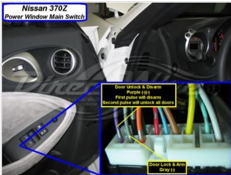
Wiring Photo and Notes: Factory Alarm Disarm
