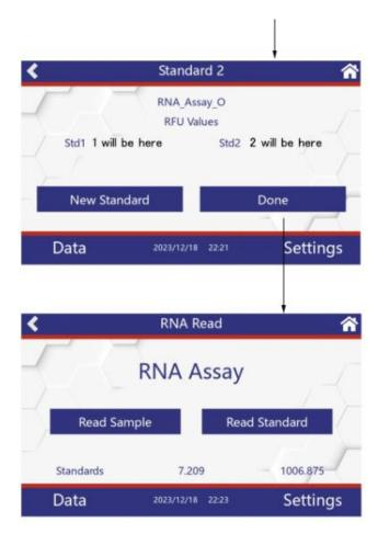
3. Tap the **Read Sample** button, slide small round icon to enter the original sample volume, tap **ng/mL** to choose RNA concentration Unit, insert an unknown sample, close the lid and quantify it using **Read tube** button.
