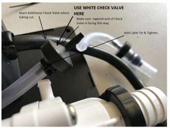
Fit new Check Valve to cut end as shown. Make sure tapered end faces correct direction, add cable ties & tighten.
