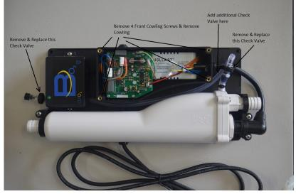
DISCONNECT POWER cord to UV/Ozone Unit and leave filtration pump RUNNING (this will prevent water leaking from the unit while the tubing is disconnected). Undo 4 Cowling Screws & Remove Cowling. Replace Check Valve on left hand side. Replace internal check valve and add additional back up check valve as follows:
