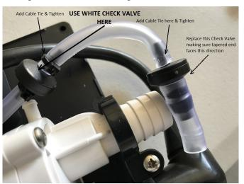
Replace existing Check Valve with new one making sure tapered end faces correct direction. Add cable ties & tighten.
