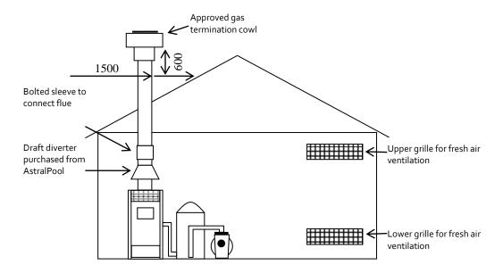
An indoor draught diverter must be purchased from AstralPool and fitted to unit in accordance with AstralPool's Instructions and Installation Codes before the heater can be enclosed.
