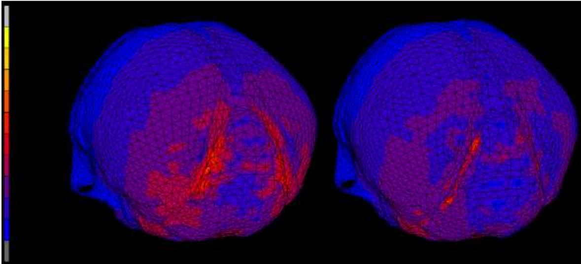
Figure 15: Von Mises stress distribution in occipital region of skull for each support type: (a) mattress and (b) foam pillow. Lower stresses were predicted for the foam pillow support condition.
