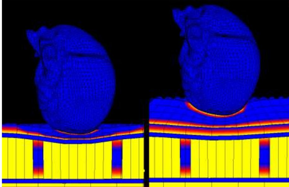
Figure 13: Cross-sectional view of contact areas between skull and each support material: (a) mattress and (b) foam pillow. Yellow regions indicate contact areas between the various bodies in the model.
