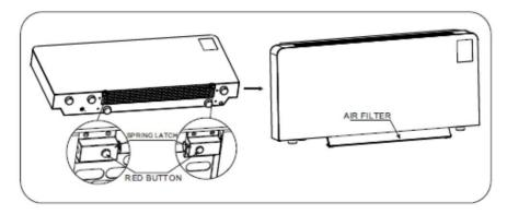
To remove the filter, press the two single red buttons to the left and right of the filter guard. This will allow the filter to drop down.
