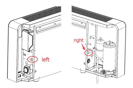
Connect the condensate hose (16mm diameter) and ensure that the water is flowing downhill with no kinks or blockages. You have the choice of fitting the drain on the right or left side. The hose on the right is pre-fitted, if you wish to change to the left, remove the bung from the left and swap it with the hose on the right.
