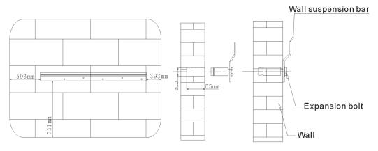
Using the enclosed, drill five holes for the wall mounting bracket and secure using the expansion bolts. When wall-mounting, the wall and the bracket level must be true or water will leak from the dehumidifier.
