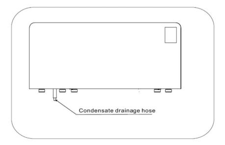
If you wish to move the drain to the other side, then you can do so by removing the side covers - this should only be done by a qualified electrician and only when the units power supply has been turned off and isolated.
