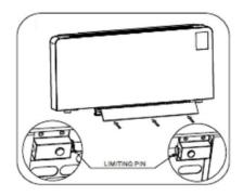
Wash the filter in water and allow to dry fully before refitting. Once the filter is dry reinsert and allow the safety springs to clip back into place on the right and left.
