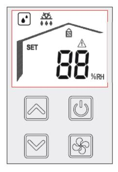
When the dehumidifier is turned on the display will show 88 and then the program version number for ten seconds. This is to allow the relative humidity sensor to sample the air and to take a reading. The display will dim after 90 seconds of no keys being pressed.
