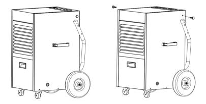
2. Rotate the pushing handle, aim it at the hole site, then tighten the hand-screws.
