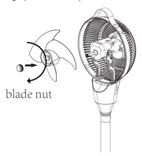
3. Clean the fan blades and the internal part of the fan using a soft dry cloth. Reverse the procedure to put the air circulator back together. Make sure the locking cap is tightened securely.
