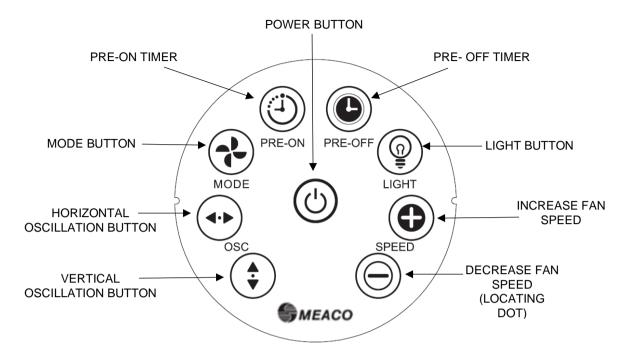
The following functions are only available via the remote control. All other buttons on the remote-control work in the same way as the control panel (see pages 6 and 7). The remote control has a range of approximately three metres. Before using the remote control, remove the plastic tab.
