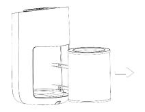
2. Push the filter down and twist it clockwise to remove.
