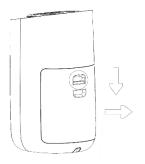
1. Open the filter door by squeezing the button on the door to release.
