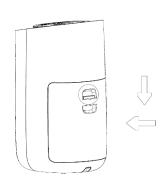
5. Put the filter door back in place – squeeze the button on the door to reinsert.
