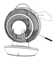
2. Squeeze four locks to pull away the front guard. At the front of the fan blades there is a locking cap – unscrew the cap in a clockwise motion to remove the fan blades.
