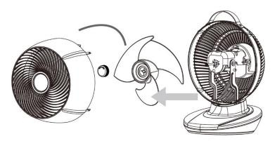
3. Clean the fan blades and the internal part of the fan using a soft dry cloth. Reverse the procedure to put the fan back together. Make sure the locking cap is tightened securely.
