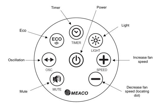
The following functions are only available via the remote-control. All other buttons on the remote-control work in the same way as the control panel (see page 4). The remote control has a range of approximately three metres. Before using the remote control, please remove the plastic tab.
