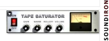
**Volume -** This knob controls the overall output level.
