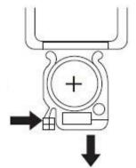
The remote control supplied with this appliance uses a CR2025 coin type battery.
