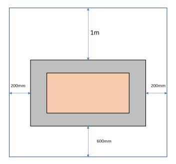
The wall bracket must be fitted horizontally and the cable routed to the bottom right of the heater. A distance of 600mm from bottom of heater to floor is recommended for optimum viewing of fuel bed. Mark the top four screws fixing positions on wall in accordance with the pre-drilled holes in the wall bracket.
