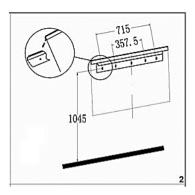
Ensure that the bracket is level by using a spirit level whilst marking out the hole positions. Drill holes with a correct size drill bit for the wall plugs.
