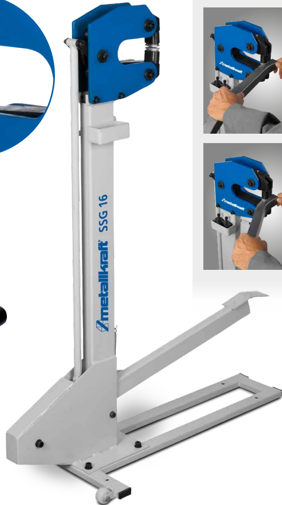
SSG 16 ▶ Force transfer to tools via foot pedal ▶ Carriage unit for ease of transport Compression jaw Stretching jaw
