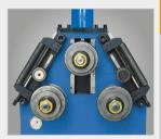
Option: special guide rollers on the sides, for angle sections
