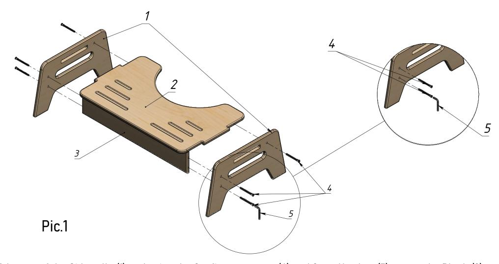
Take one of the Sidewalls (1) and using the Confirmat screws (4) and 3mm Hex key (5), screw the Plank (3) to it. Position the protruding part of a Step (2) into the hole in the Sidewall (1) and screw the parts together. Connect another Sidewall (1) using the Confirmat screws (4) to the previously assembled construction. See Pic.1
