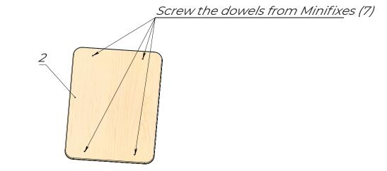
Take the Upper shelf (2) and using a Screwdriver (8), screw the Dowels from Minifixes (7) in. See Pic.3
