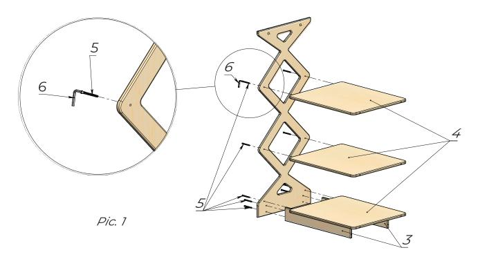
Take one of the Sidewalls (1) and using the Confirmat screws (5) and Hex key (6), connect Lower lintels (3) and the Shelves (4). See Pic.1
