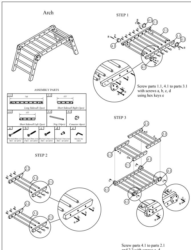
Screw parts 2.1, 2.2 to parts 3.1 with screw b using hex key e
