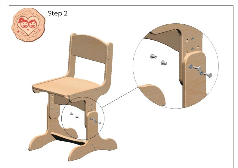
Connect two assembled structures together using the screws 2.2 and nuts 2.3 as shown on the picture.
