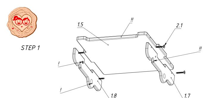
Take the Platform (1.5) and screw it together with the Connectors (1.7; 1.8) using the Confirmat screws (2.1) as shown on the picture.
