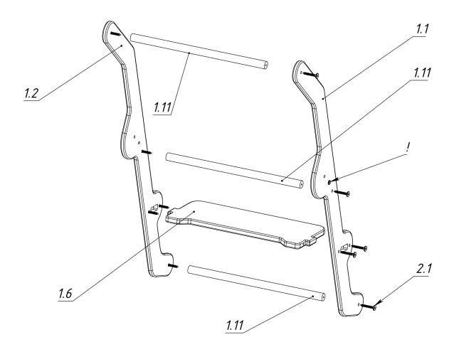
Take the outer planks (1.1; 1.2) and position them as shown on the picture. Now take the Long nogs (1.11) and insert them between the Outer planks from top and bottom with flat head screws (2.2). Do not tighten the screws.
