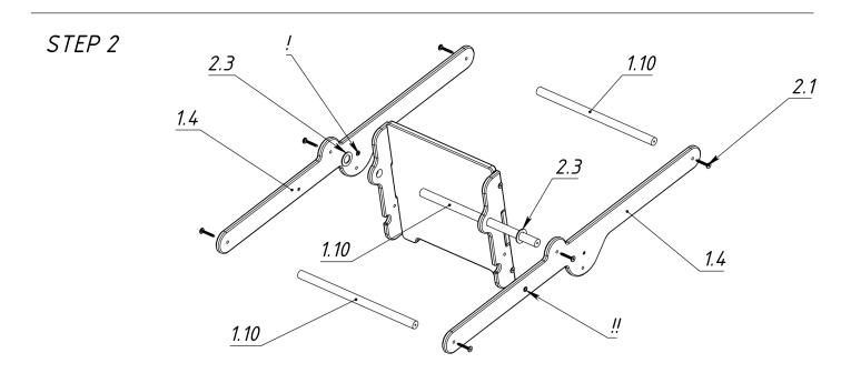
Take the structure assembled in Step 1 and insert the Short nog (1.10) through the holes in the Connectors. Put the Shims (2.4) on both ends of the nog.
