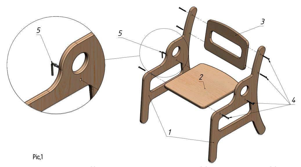
Take one of the Sidewalls (1) and using the Confirmat screws (4) and 3 mm Hex key (5), connect the Seat (2) and a Backrest (3).
