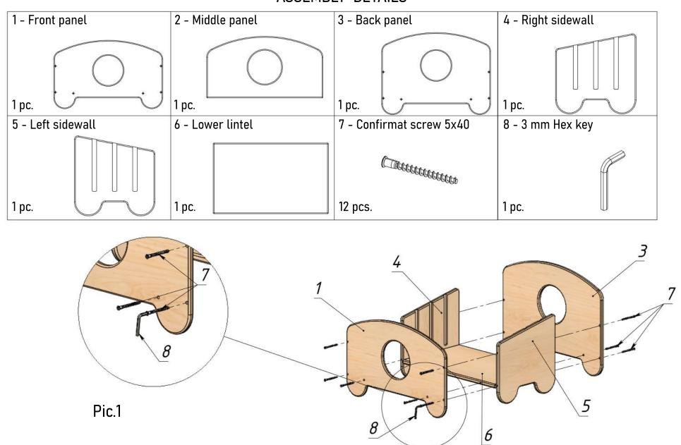
Take the Front panel (1) and using the Confirmat screws (7) and Hex key (8) connect the Right sidewall (4), Left sidewall (5), and Lower lintel (6) sequentially. Then connect the Back panel (3) using the Confirmat screws (7) in a same way, See Pic.1
