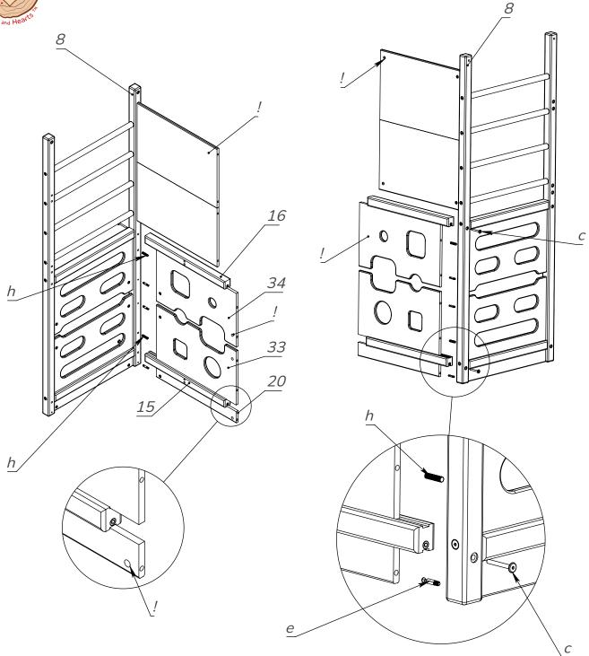
Take the stand (8) and screw the minifix dowels (e) using the screwdriver (k). Plug the wooden dowels (h) into the stand (8).
