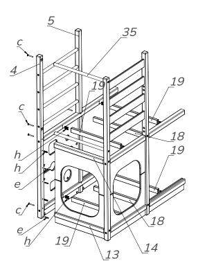
Take the stand (4) and insert the minifix dowels (e) using the screwdriver (k).
