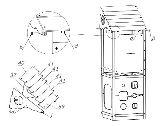
Connect the details (39), (40), and (41) to the details (37) and (38) using the screws (f) and a screwdriver (k).
