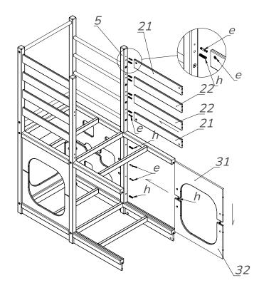
Take the stand (5) and screw the minifix dowels (e) in, using the screwdriver (k). Plug the wooden dowels (h) into the stand (5).
