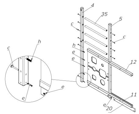
Screw the minifix dowels (e) into the stands (4, 5) using the screwdriver (k). Plug the wooden dowels (h) into the stand (4).
