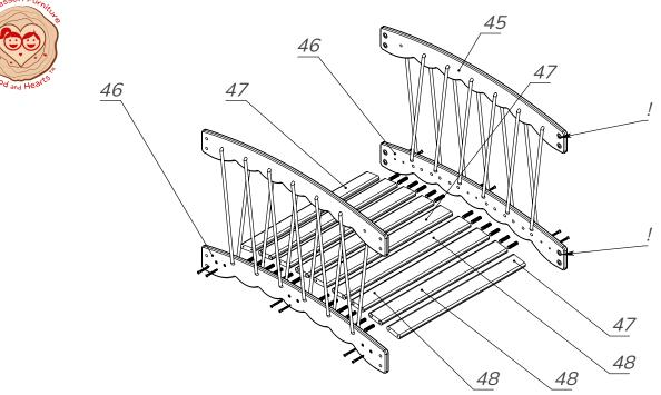
Take the detail (48) and Plug the wooden dowels (h) from the both sides. Assemble the construction as shown on the picture, the detail (46) is to be connected to the detail (47) using the screws (g) and a hex key (j). ! - Grooves should be inside
