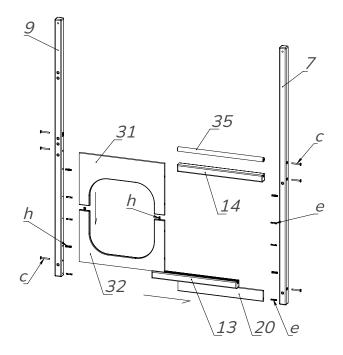
Take the stand (7) and (9) and screw the minifix dowels (e) using the screwdriver (k). Plug the wooden dowels (h) into the stand (7) and (9).
