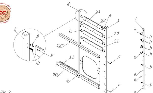
Screw the minifix dowels (e) into the stands (1, 2) using the screwdriver (k). Plug the wooden dowels (h) into the stands (1, 2).
