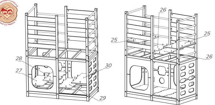
Connect the details (27), (28), (29) on the first floor, and the details (25) and (26) on the second floor using the screws (f) and a screwdriver (k) as shown on the Pic. 10.
