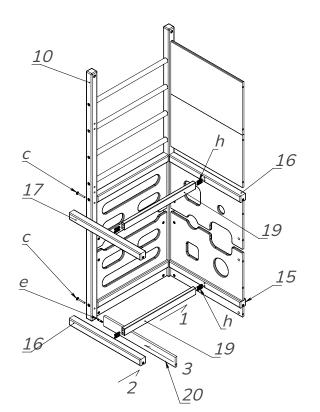
Take the stand (10) and screw the minifix dowels (e) using the screwdriver (k). Take the detail (19) and Plug the wooden dowels (h) from the both sides and install the details (15) and (16). [1]
